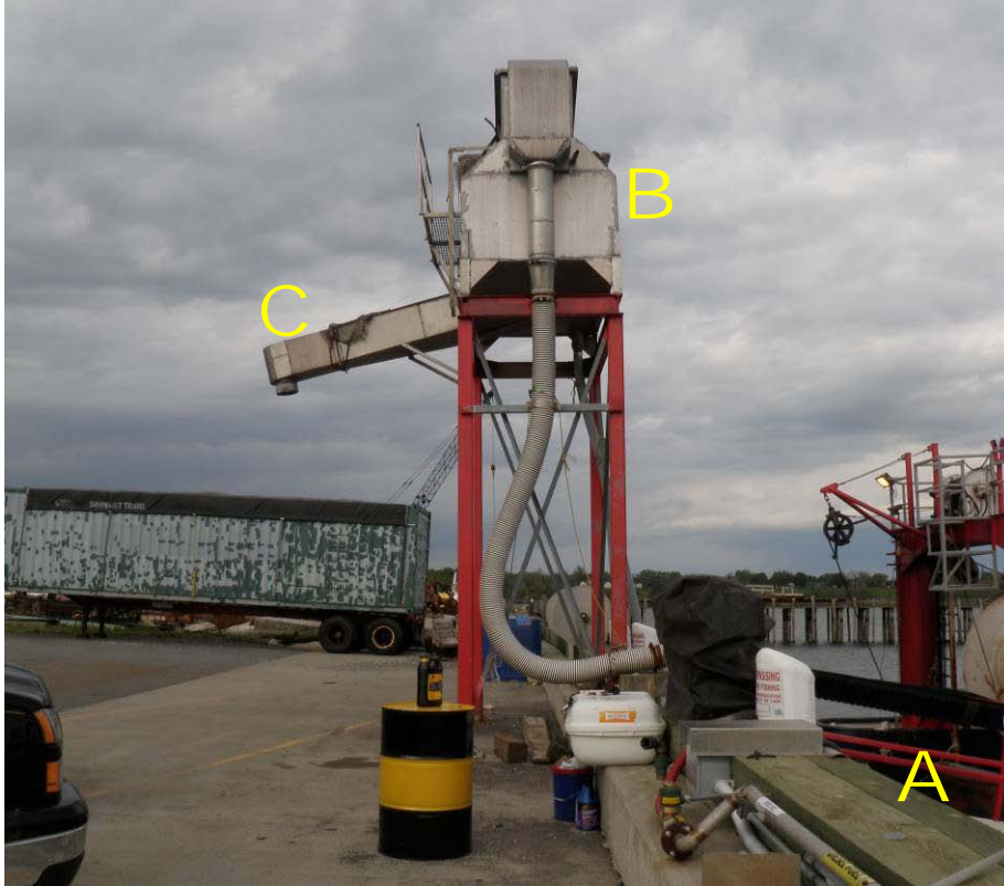
Figure 12. At this port herring are unloaded from the vessel, into tubes on the dock (A), up through another tube and into a dewatering box (B). Trucks drive under the end of the dewatering box (C) and fish are dumped into containers or the truck itself (not pictured).
